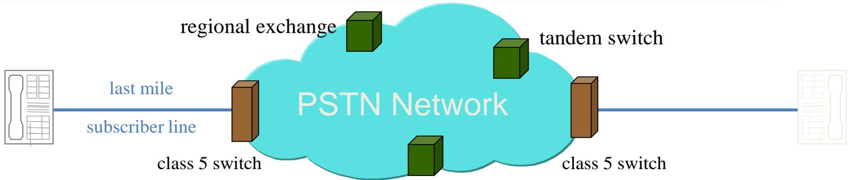
Analog voltages and copper wire used only in “last mile”,
